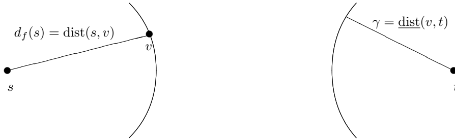
FIGURE 2. Pruning using implicit bounds. Assume v is about to be scanned in the forward direction, has not yet been scanned in the reverse direction, and that the smallest distance label of a vertex not yet scanned in the reverse direction is \gamma . Then v can be pruned if \bar{r}(v) < d_f(v) and \bar{r}(v) < \gamma .
