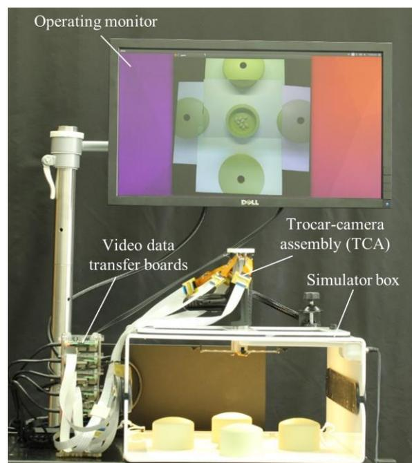
**Figure 3.** Demonstration setup. The TCA is inserted into the simulator box. Video data from five cameras are transferred to a computer through video data transfer boards and then the stitched video is shown on the operating monitor.
