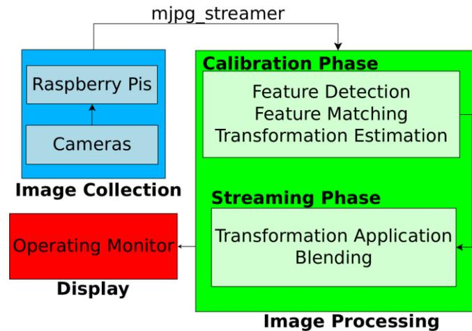
Figure 4. Flowchart of the real-time video stitching process.
