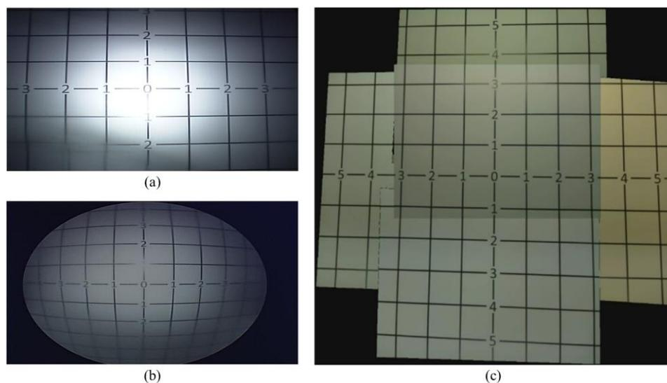
**Figure 6.** FoV measurement using grid lines printed on a paper sheet. Captured images from (a) a 10 mm  $0^\circ$  laparoscopic camera, (b) a 5 mm  $0^\circ$  laparoscopic camera, and (c) the TCA. The TCA can cover larger FoV compared with commercial laparoscopic cameras. Note the distortion in the view acquired from the 10 mm  $0^\circ$  laparoscopic camera (a) and the 5 mm  $0^\circ$  laparoscopic camera (b).
