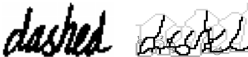
Figure 4. Segmentation heuristics using skeleton endpoints (the word is: "dashed")
