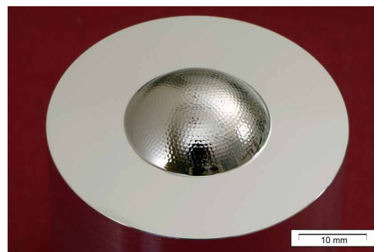
Fig. 7. A finished freeform microlens array mold insert containing 1,219 single spherical lenslets.
