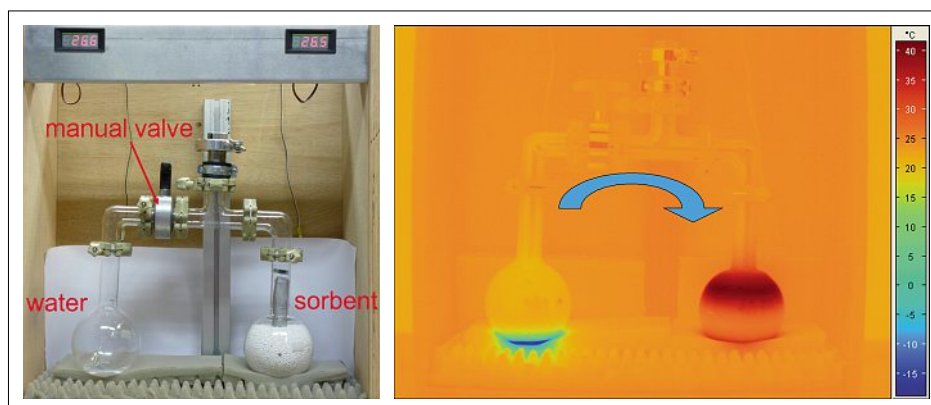
Fig. 3. Experimental setup for the illustration of the working cycle ( cf. Fig. 2) in a TDC or AHP. The flasks with water and empty sorbent material are under vacuum. Left: Before opening the manual valve. Right: Infrared photograph a few minutes after opening of the valve with indication of the different temperatures \sim\text{--}5 °C in the water flask (with ice formation) and \sim\text{40} °C in the sorption material.
