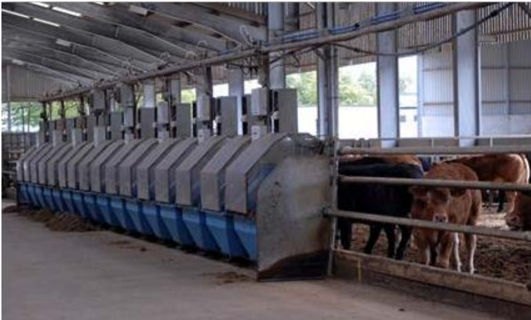
Figure S1. Detail of the Hoko feeders used in the study to assess feeding behaviour and methane emissions. The blue part contains the feed and records each time a steer accesses the feeder. On top of it, the transparent cover contains the gas exhaled, which was vacuumed towards a gas chromatograph.
