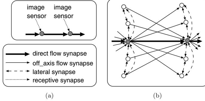
Fig. 2. A close view of four types of inter-neural connections in Fig. 1. (a) Side view of the connection structure of two neurons on an axis. (b) Top view of the connection structure of two neurons on an axis.
