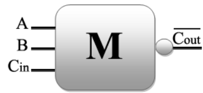
Figure 6. Producing \overline{C_{out}} by using a 3-input Majority-not gate.
