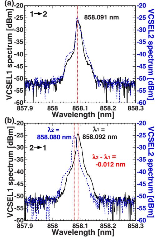
FIG. 6. (Color online) Experimental result of optical spectra of the  $y$ -mode intensity of VCSEL 1 and 2 when an optical isolator is inserted in the optical path of the two VCSELs to obtain unidirectional coupling (a) from VCSEL 1 to 2 and (b) from VCSEL 2 to 1. The wavelength of the solitary VCSEL 1 is longer than that of the solitary VCSEL 2. Injection locking is achieved in (a), but not in (b). Solid (black) curve, VCSEL 1; and dotted (blue) curve, VCSEL 2.
