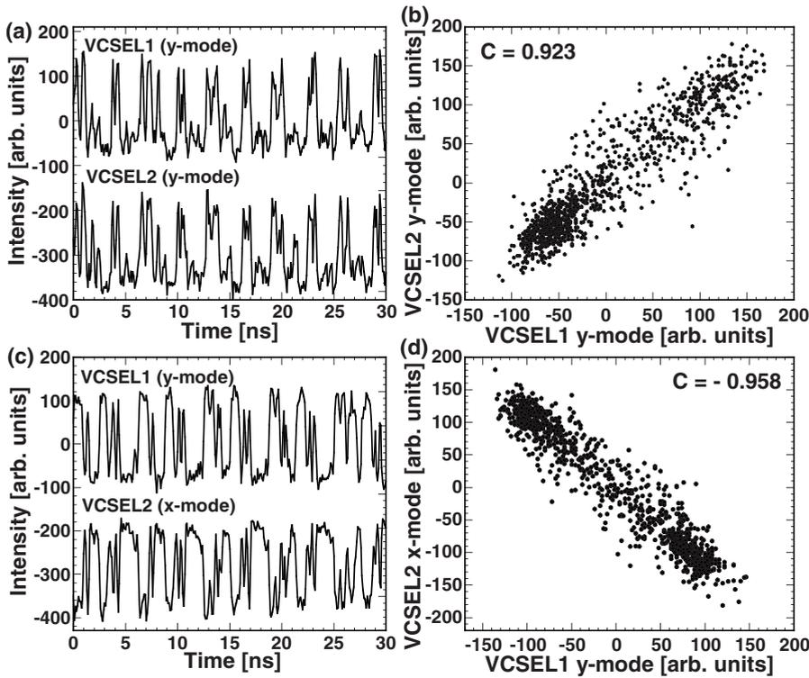
FIG. 3. Experimental result of temporal wave forms and correlation plots for (a),(b) y mode of VCSEL 1 and y mode of VCSEL2, and for (c),(d) y mode of VCSEL 1 and x mode of VCSEL 2. The temporal wave form of VCSEL 2 is shifted with respect to VCSEL 1 by the one-way coupling delay time ( $\tau=3.2$  ns) to obtain the optimal synchronization. The cross correlation is (b) 0.923 and (d)  $-0.958$ , respectively.
