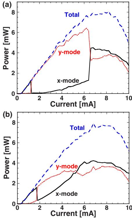
FIG. 1. (Color online) Light power–injection current ( $L$ - $I$ ) characteristics for (a) VCSEL1 and (b) VCSEL2. Solid (black) curve,  $x$ -mode intensity; dotted (red) curve,  $y$ -mode intensity; and dashed (blue) curve, total intensity.
