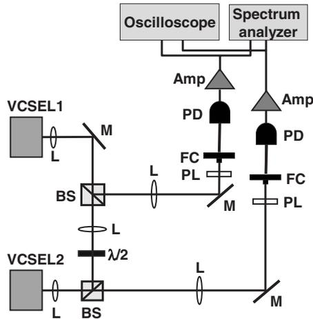
FIG. 2. Experimental setup for chaos synchronization in two mutually coupled VCSELs. Amp, electronic amplifier; BS, beam splitter; FC, fiber collimator; L, lens;  $\lambda/2$ , half-wave plate; M, mirror; PD, photodetector; PL, polarizer.
