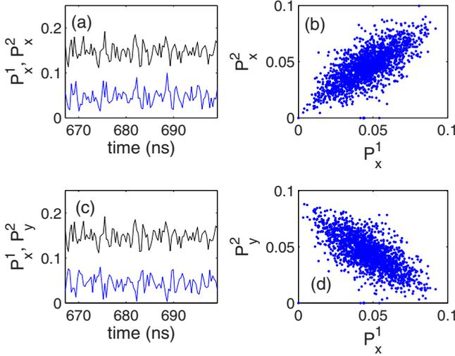
FIG. 7. (Color online) Numerical result of temporal wave forms and correlation plots for (a),(b)  $x$  mode of VCSEL 1 and  $x$  mode of VCSEL 2, and for (c),(d)  $x$  mode of VCSEL 1 and  $y$  mode of VCSEL 2. The temporal wave form of VCSEL 2 is shifted with respect to VCSEL 1 by the one-way coupling delay time ( $\tau=3.2$  ns) to obtain the optimal synchronization.
