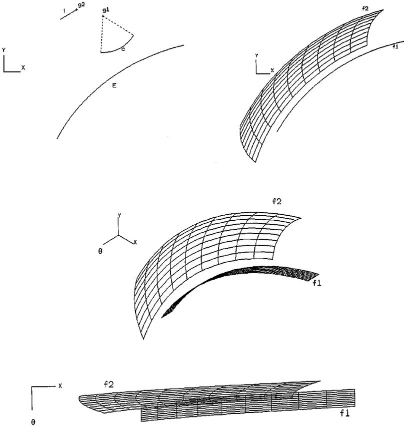
**FIG. 2.6.** Two examples of  $c$ - $E$  contact. f1:  $c$ - $E$  contact configurations when  $g_1$  (center of arc  $c$ ) is the reference point of  $c$ . f2:  $c$ - $E$  contact configurations when  $g_2$  is the reference point of  $c$ . Both have the same reference vector  $l$ .
