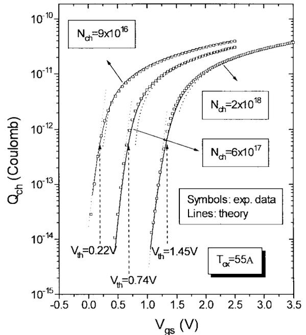
Fig. 1. Channel charge model fits the measurement data taken from devices with different  $N_{ch}$  well, and also can match the simulation results (dashed lines) from the model equations (1) and (6) in strong inversion and subthreshold regions respectively. The model covers weak, moderate, and strong inversion regions of NMOSFET's.
