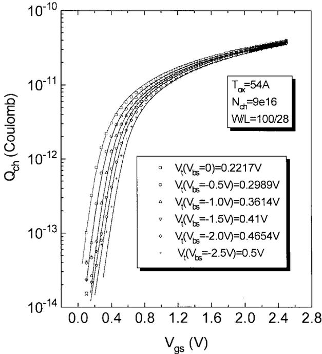
Fig. 3. Channel charge model fits the measurement data well for different substrate body biases of NMOSFET.
