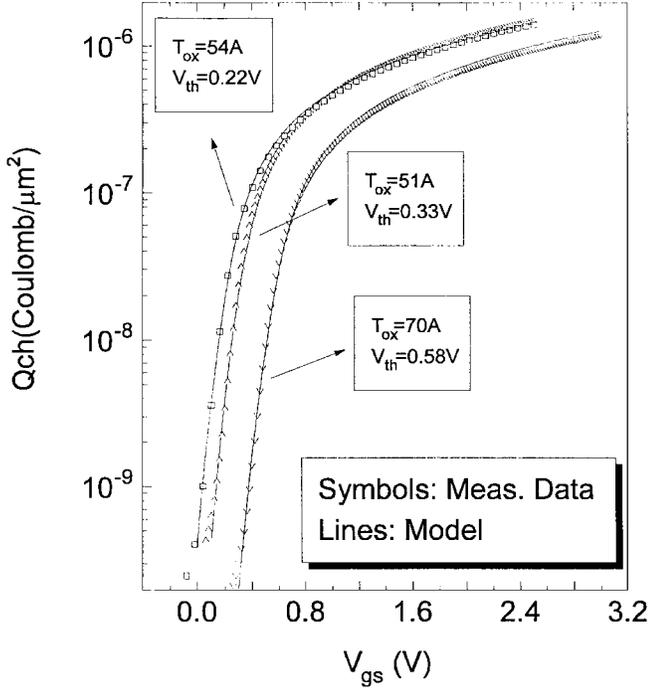
Fig. 2. Channel charge model fits the measurement data taken from devices with different gate oxide thickness of NMOSFET's.
