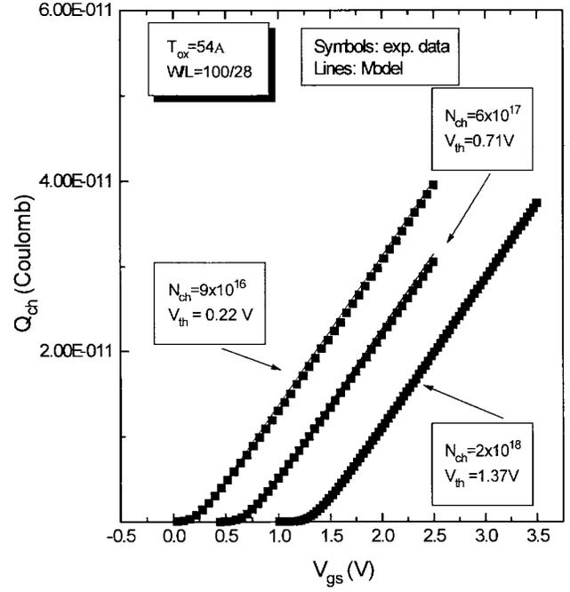
Fig. 4. Same data used in Fig. 1 is plotted in linear scale to show the model accuracy in strong inversion for different devices with different oxide thickness.
