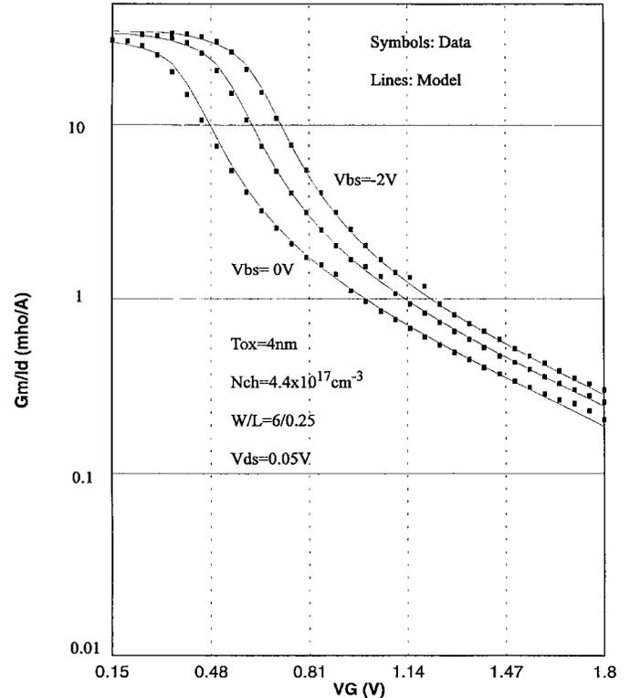
Fig. 5.  $I-V$  model that implements the presented channel charge model shows excellent continuity characteristics as well as fits the measurement data of  $g_m/I_d$  well.  $g_m/I_d$  is an important parameter for model continuity and analog design merit test.
