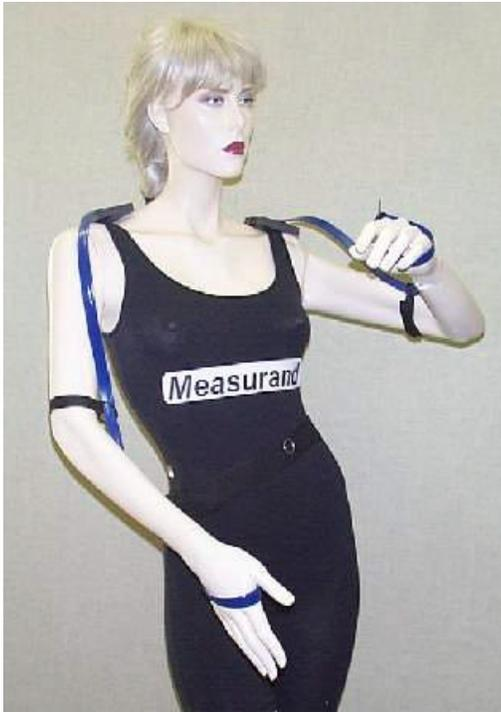
**Figure 7** Two SHAPe TAPEs™ for robotic control or motion capture.
