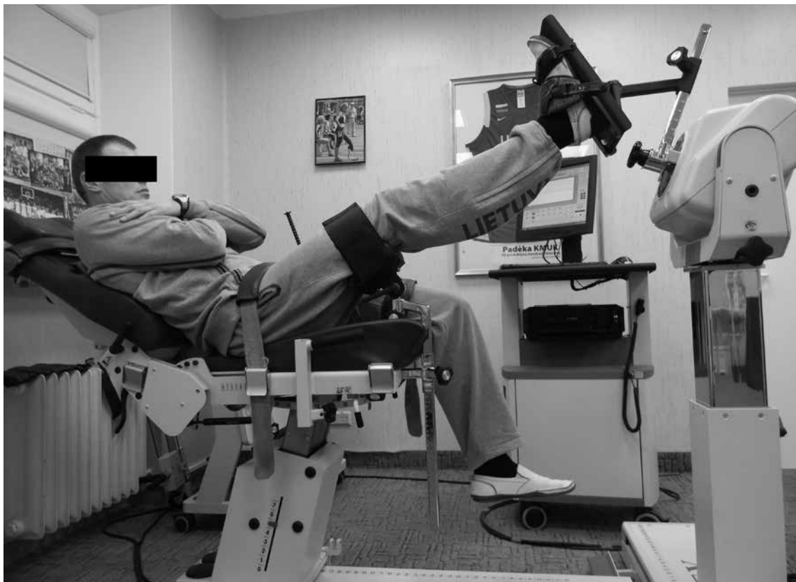
Figure 1 — Patient positioning on the dynamometer.
