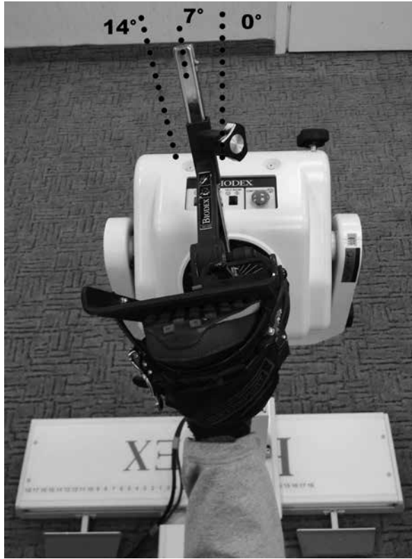
Figure 2 —Dynamometer footplate position set at 7° of inversion (view from above).
