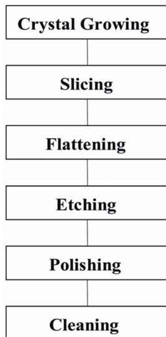
Figure 1 Major processes for 300 mm silicon wafer manufacturing
