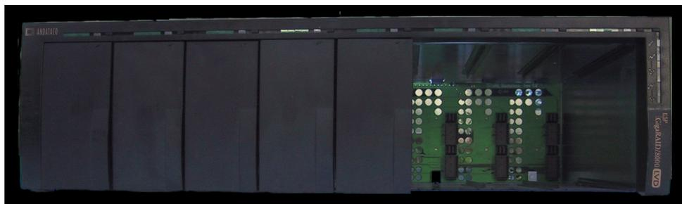
**Figure 5: A shelf with five bricks inserted and three empty spaces.**
