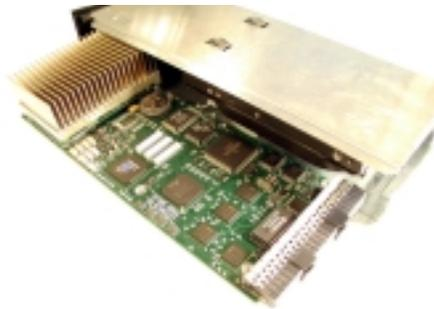
**Figure 2: A ROC-1 brick.** The processor board is shown partially removed from the canister, and with its disk removed.
