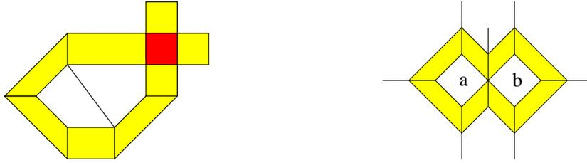
Figure 4: Quadrilaterals forming part of a self-intersecting dual cycle (left) and an example of a simple dual cycle (right) where the enclosed quadrilaterals  $a$  and  $b$  are disconnected with respect to the dual graph (although they share a primal vertex).
