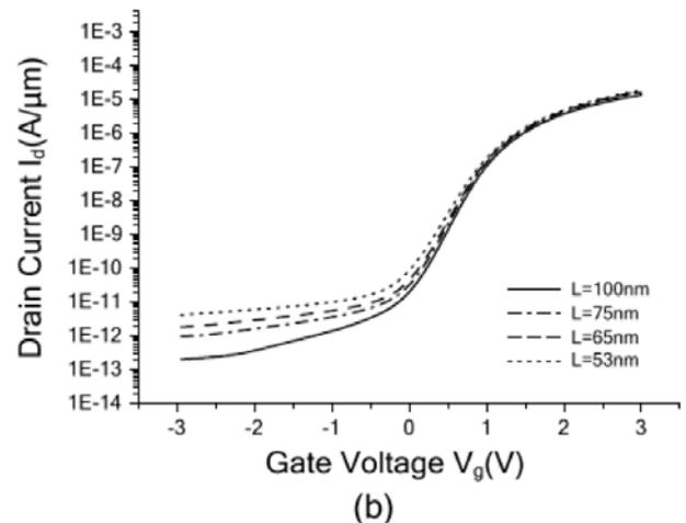
**Figure 8**  $I_d$ - $V_g$  characteristics at  $V_d = 1.2$  V for (a) and SOI (b) Single-GB TFT using the calibrated energy balance model. The subthreshold degradation in the SOI device becomes severe at the increased drain bias whereas the single-GB TFT shows good DIBL immunity
