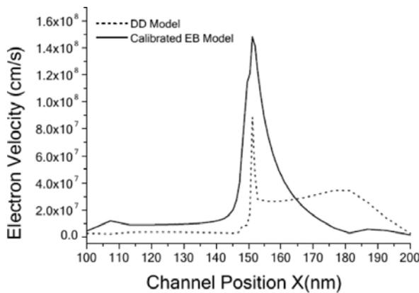
This is as a direct consequence of the velocity overshoot effect and this is the reason for the increased drain current. The  $I_d-V_d$  characteristics are shown in Figure 6. These provide further clear illustration of the larger drain currents that result when using the EB model.
