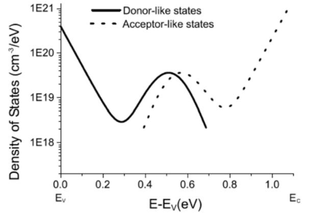
As it is widely accepted that the trap density distribution contains exponential band tails at the valence and conduction band edges, when deciding on a suitable distribution the main qualitative choice is whether to include the mid-gap states as additional exponential terms
