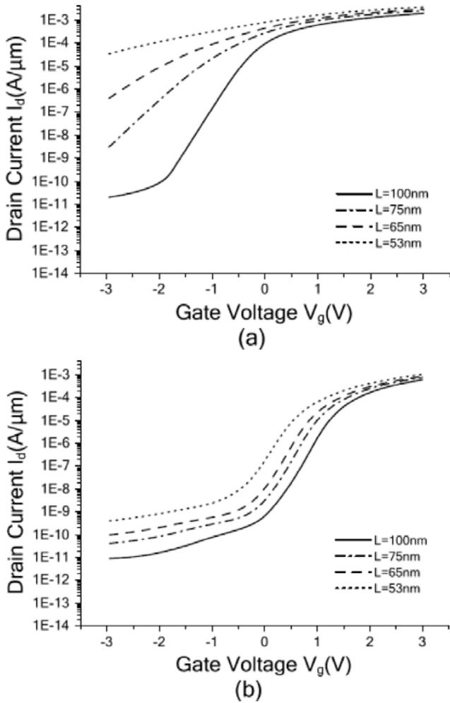
When  $V_d = 0.01$  V, the SOI MOSFET shows better short channel behaviour than when simulated in Walker et al.). This is because the LDD doping profile reduces the electric field at the drain edge and therefore reduces the DIBL. However, at the higher drain bias of  $V_d = 1.2$  V, the SOI MOSFET shows poor DIBL immunity, with subthreshold slope and leakage currents becoming unacceptable as the channel length of 53 nm is approached.
