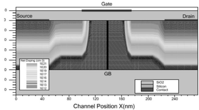
We choose to limit the maximum channel length used in this study to  $L = 100$  nm. This is because 100 nm is close to the limit where the DD model is thought to become inaccurate and is of a magnitude in the order of the size of grains that are typically obtained by SPC of deposited a-Si.
