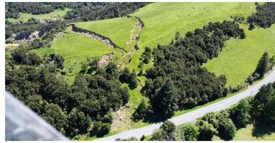
(a) Ruptured ground with increased landslide risk to the road. Photo credit: Aurecon, 2016
