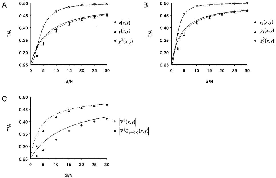
**FIG. 5.** The effect of  $S/N$  on the noise bias:  $T/A$  vs  $S/N$  for  $q=0.25$  and  $\varepsilon=1/16$ . The symbols mark experimental values, the curves were computed from the high  $S/N$  approximation. Part (A) shows the results for the  $\Delta$ -based filters; (B) shows the results for the  $\Delta_{\text{Sobel}}$ -based filters. The solid lines represent  $e(x, y)$ , the dotted  $g(x, y)$  and the dashed  $g^2(x, y)$ .
