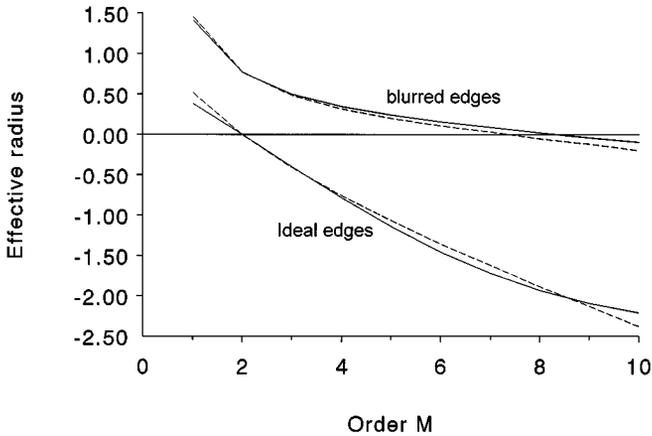
**FIG. 3.** Effective filter radius  $r_{\text{eff}}$  as a function of the order  $m$  of the filter for Sobel and simple first derivatives: ideal edges and blurred edges.
