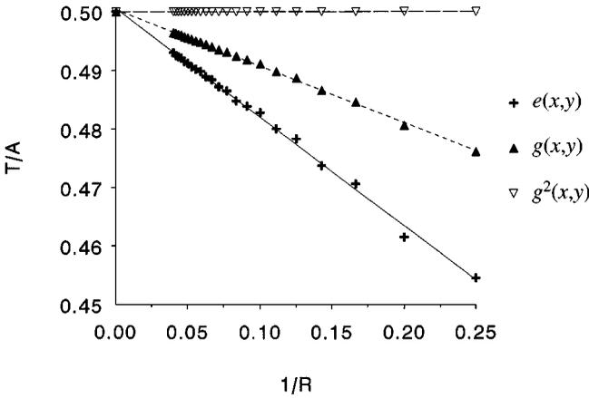
**FIG. 2.** Curvature bias as a function of object size:  $T/A$  as a function of  $1/R$  for circles with radii ranging from 4 to 25 pixels, for the three  $\Delta$ -based gradient filters. The effective radius  $r_{\text{eff}}$  can be derived from the slope of the least squares linear fit.
