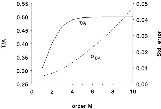
**FIG. 8.**  $T/A$  and its standard error  $\sigma_{T/A}$  as a function of the order  $m$  of edge detectors of the form  $g^m(x, y)$  for  $q = 0.25$ ,  $S/N = 10$ , and  $\varepsilon = 1/16$ . The solid line denotes  $T/A$ , the dotted  $\sigma_{T/A}$ . As  $m$  increases, the bias is reduced at the expense of a higher standard error.
