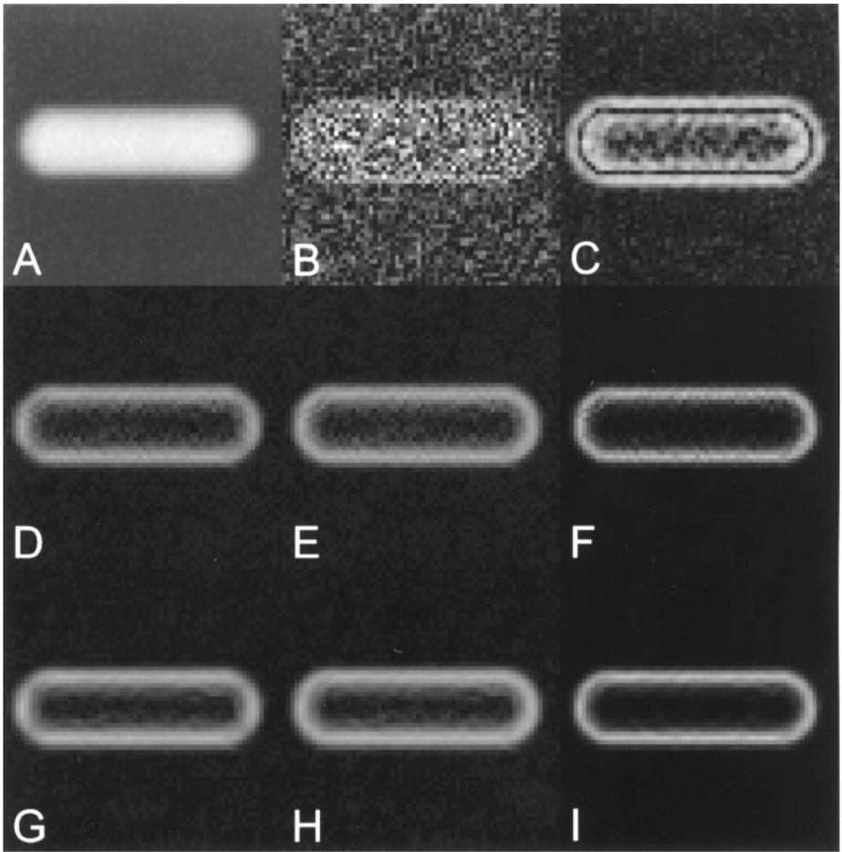
**FIG. 1.** The effect of 8 different gradient on a simulated shape of a bacterium (A)  $e(x, y)$ ; (B)  $g(x, y)$ ; (C)  $g^2(x, y)$ ; (D), (E), and (F) same as (A), (B), and (C), respectively, but using Sobel filters instead of  $\Delta(x, y)$ .
