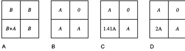
**FIG. 9.** Discrete curvature bias of a  $90^\circ$  corner for the three  $\Delta$ -based filters: (A) shows the grey levels at the pixels at the corner point; (B) shows the values of  $e(x, y)$ , yielding a local threshold of  $T = B + A/3$ ; (C) shows  $g(x, y)$ , yielding  $T = B + A/2.41$ ; (D) shows  $g^2(x, y)$ , yielding  $T = B + A/2$ .
