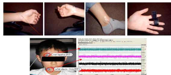
Figure 2: The attachment of electrodes for measure of physiological signals. (above: ECG and EDA, below: facial EMG)
