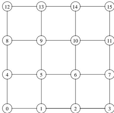
Fig. 1. The 2-dimensional 4-ary array  $A_4^2$ .
