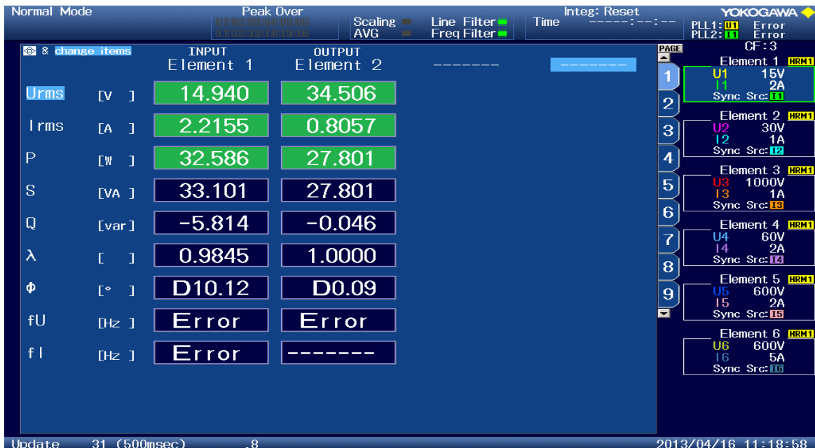
Fig. 17: Input and output values of modified cuk converter (85.3% duty cycle)
