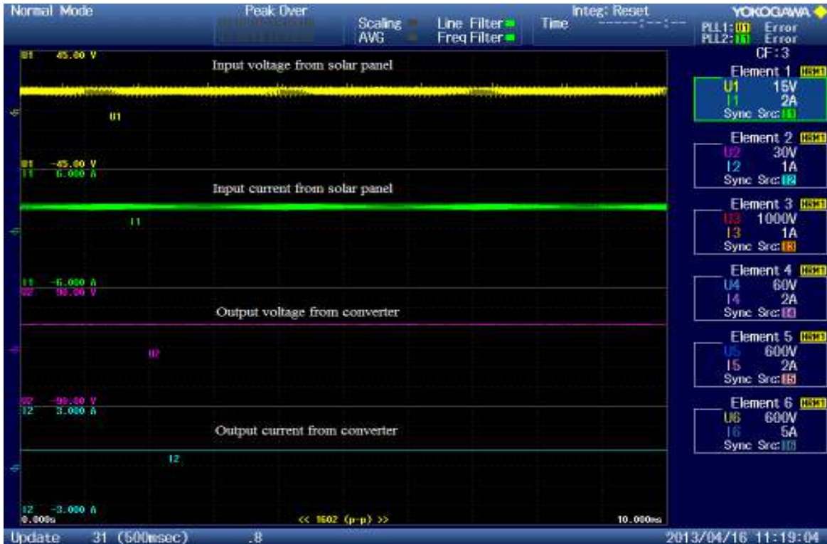
Fig. 16: Voltage and current waveforms of modified cuk converter for 85.3% duty cycle
