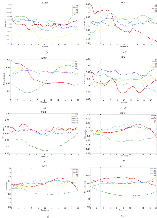
Fig. 8. Difference between the ZTD of IGS station and the forecast ZTD data of ECWMF on the day mainly from day 300 to 304 in 2012. The dotted lines represent the epoch of the earthquake. At site 7-WHIT, ZTD on day 303 was missing and thus was substituted by ZTD on day 305.
