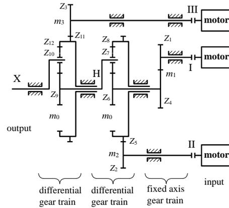
Figure 3. The diagram of TR-B triple-redundancy transmission system
