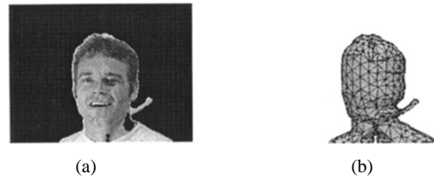
Fig. 5. Sample results for (a) automatic object segmentation considering cast shadows and (b) automatic 3-D shape estimation corresponding to the sample image in Fig. 4(a).
