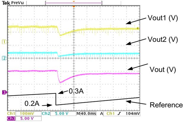
Fig. 15. MIC output voltages  $V_{out1}$ ,  $V_{out2}$  and overall voltage  $V_{out}$  (color online).
