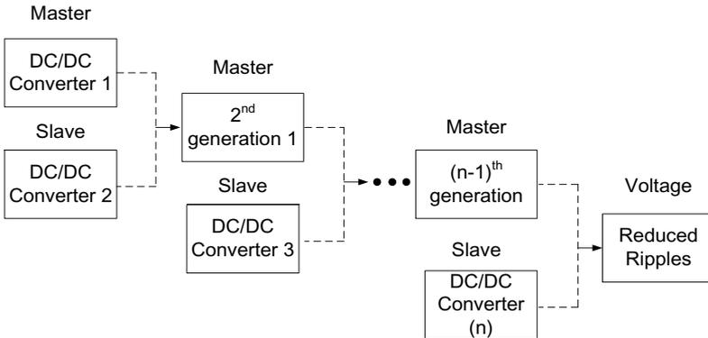
Fig. 7. The proposed interleaving technique to reduce dc-bus voltage-ripples of “ $n$ ” series MICs scheme.
