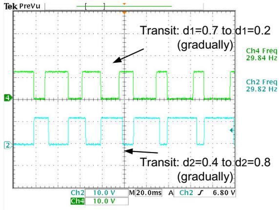
Fig. 17. Gate signals of two converters in transit test 2 (color online).
