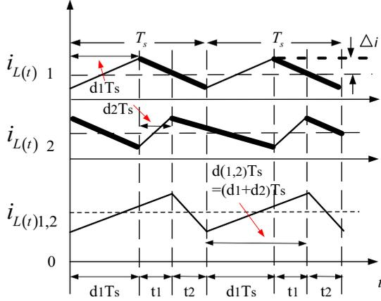
Fig. 6. Two inductor currents from each MIC  $i_{L1}$ ,  $i_{L2}$ , and the second generation current obtained virtually from the sum of  $i_{L1}$  and  $i_{L2}$  (color online).
