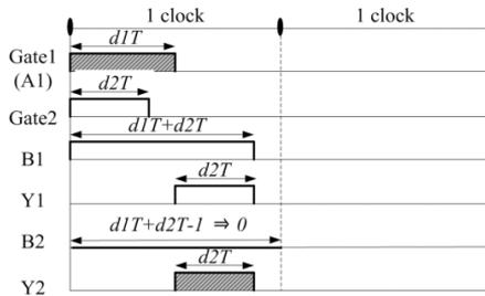
Fig. 9. Operation of the switching signals ( $d_1 + d_2 \leq 1$ ).
