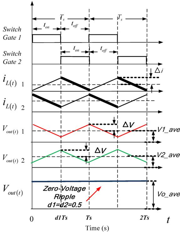
Fig. 5. Key waveforms of the proposed interleaving operation between series boost MICs ( $d_1 = d_2 = 0.5$ ) (color online).
