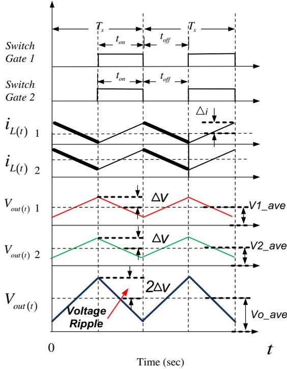
Fig. 4. Key waveforms of typically uncontrolled series connected MICs, ( $d_1 = d_2 = 0.5$ ) (color online).
