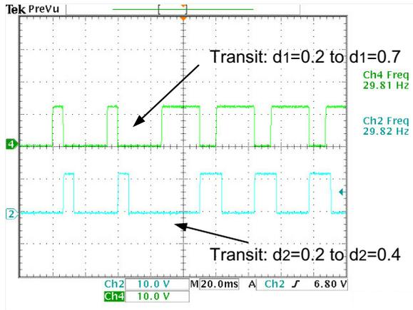
Fig. 16. Gate signals of two converters in transit test 1 (color online).
