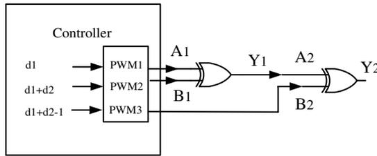
Fig. 8. Implementation of the proposed switching technique.
