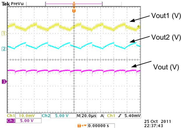
Fig. 14. MIC output voltages  $V_{out1}$ ,  $V_{out2}$  and  $V_{out}$  (color online).
