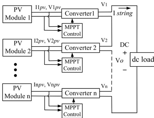
Fig. 2. Series-connect MICs of PV-converter-dc load scheme.
