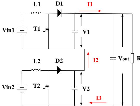
Fig. 3. Series connected two boost-type MICs scheme (color online).
