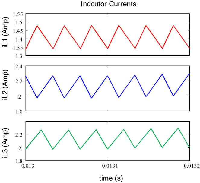
Fig. 11. Inductor currents of series converters:  $i_{L1}$ ,  $i_{L2}$  and  $i_{L3}$  (color online).
