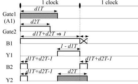
Fig. 10. Operation of the switching signals ( $d_1 + d_2 > 1$ ).
