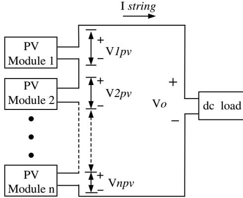
Fig. 1. Series connected PV panel string.
