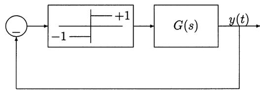
Fig. 1. Block diagram of a nonlinear oscillator.
