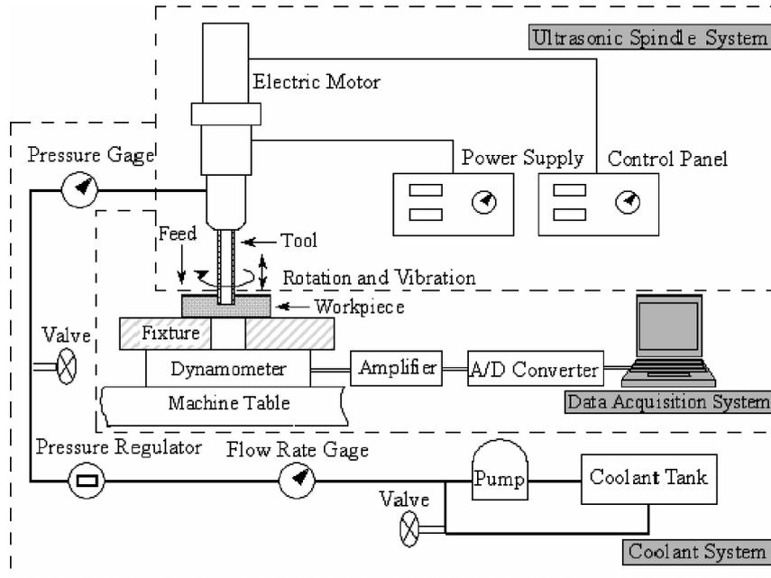
Mobilemet<sup>®</sup> S122 water-soluble cutting oil (MSC Industrial Supply Co., Melville, NY, USA) was used as the coolant (diluted with water at 1–20 ratio).
