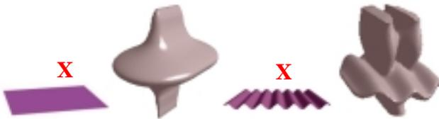
Figure 20: The plane used as the abscissa figure 19 is replaced by a wavy field. The PROFILE extrusion become uncontrollable.
