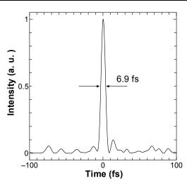
Fig. 9. Temporal time profile compensated optimally by SLM after propagation of a fiber. The pulse width (FWHM) is 6.9 fs. (Nakamura et al., 2005a)
