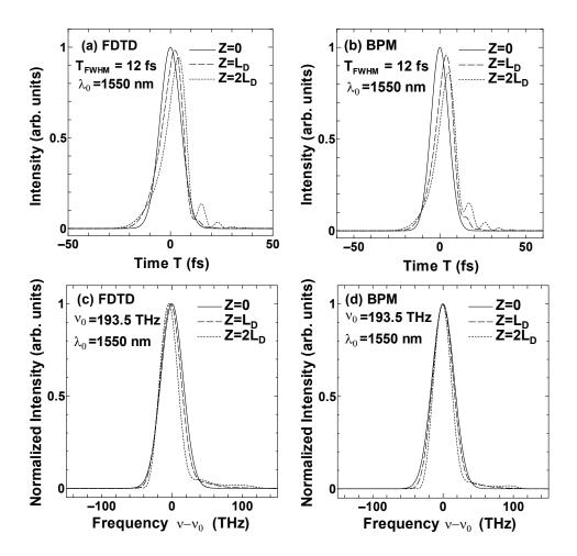
Fig. 21. (a), (b) Temporal profiles and (c), (d) spectra numerically obtained by (a), (c) the extended FDTD method and (b), (d) BPM for 12 fs, 1550 nm laser propagation through a silica fiber of up to twice the dispersion length  $L_D$ , where the laser intensity corresponds to the soliton number of 1. (Nakamura et al., 2004)
