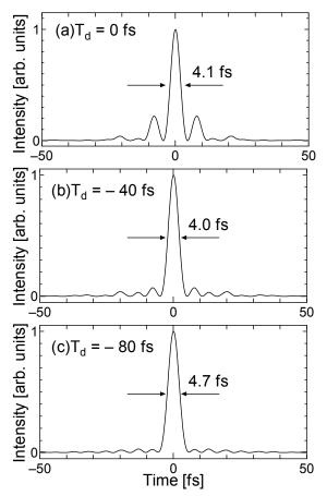
Fig. 16. Temporal profiles of transform-limited pulses obtained numerically for mixed twopulse spectra shown in Fig. 6 at center wavelengths of 795 and 640 nm after simultaneous copropagation with initial delay of (a) 0, (b) -40, and (c) -80 fs in a 3 mm silica fiber. (Nakamura et al., 2005b)
