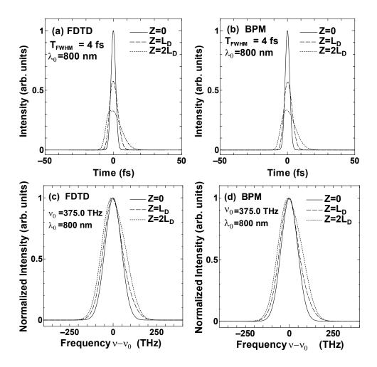
Fig. 20. (a), (b) Temporal profiles and (c), (d) spectra numerically obtained by (a), (c) the extended FDTD method and (b), (d) BPM for 4 fs, 800 nm laser propagation through a silica fiber of up to twice the dispersion length  $L_D$ , where the laser intensity corresponds to the soliton number of 1. (Nakamura et al., 2004)
