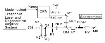
Fig. 10. Layout of the experimental setup.(Xu et al., 1999) M, silver-coated plane mirrors; R1 and R2, reflective objectives (36x); DM, dichroic mirror; NF1 and NF2, valuable optical attenuators; OPA, optical parametric amplifier.
