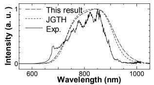
Fig. 6. Spectra after propagation of a slightly chirped 12 fs laser pulse through a 2.5-mm silica fiber, calculated by the extended FDTD (dashed line) (Nakamura et al., 2005a) and the simpler JGTH-FDTD (short-dashed line) (Nakamura et al., 2005a), and our previously reported experimental result (Karasawa et al., 2000) (solid line).
