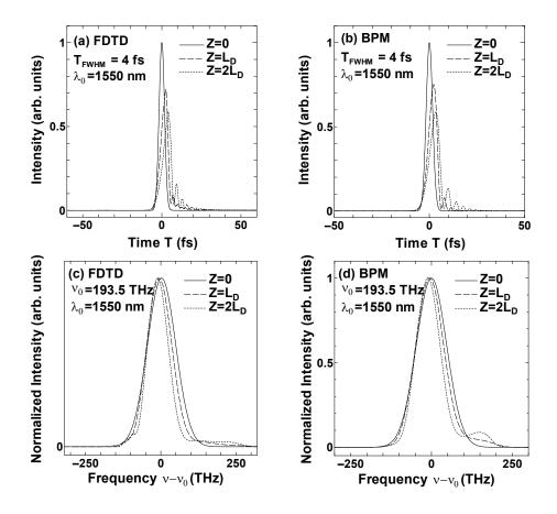
Fig. 23. (a), (b) Temporal profiles and (c), (d) spectra numerically obtained by (a), (c) the extended FDTD method and (b), (d) BPM for 4 fs, 1550 nm laser propagation through a silica fiber of up to twice the dispersion length  $L_D$ , where the laser intensity corresponds to the soliton number of 1. (Nakamura et al., 2004)
