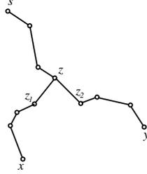
Figure 7: 2-SPT: the paths from  $s$  to  $z$ , from  $z_1$  to  $x$ , and from  $z_2$  to  $y$  are shortest paths.  $z_1$  and  $z_2$  can be reached from  $z$  by one broadcasting.
