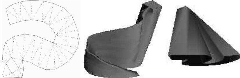
Figure 17: Example 1. Convoluted shape. Triangulation (left), reconstructed shape by our algorithm (middle), and reconstructed shape by triangular tiling (right)
