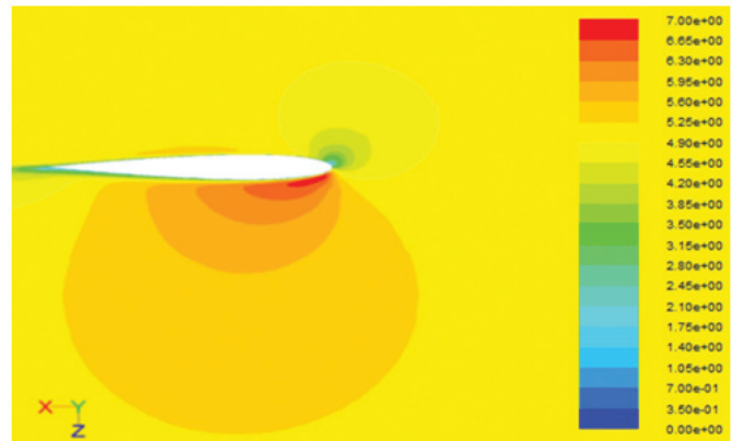
Figure 4. Velocity distribution (m/s) at 10 knots.
