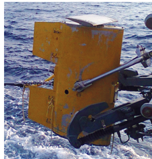
Figure 10. Towed body with depressor.
