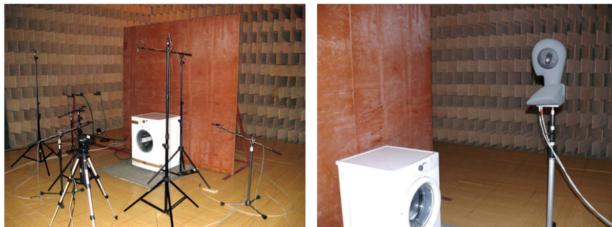
Fig. 2. Measurement of the sound power level and psychoacoustic metrics in semi anechoic chamber
