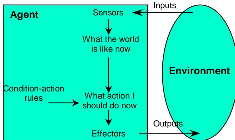
Fig. 5. The architecture of a simple reactive agent
