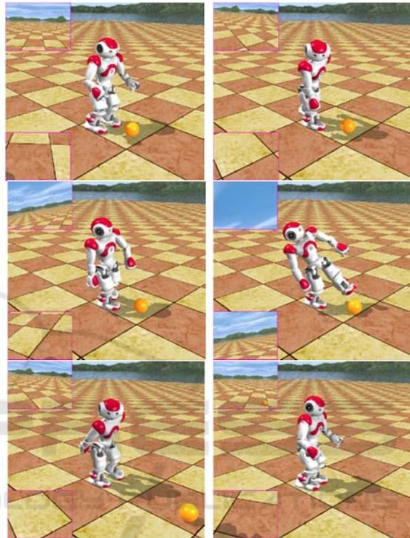
Figure 3: An example of an evolved kick, as transferred from V-REP to the Webots simulator; read from top left to bottom right.
