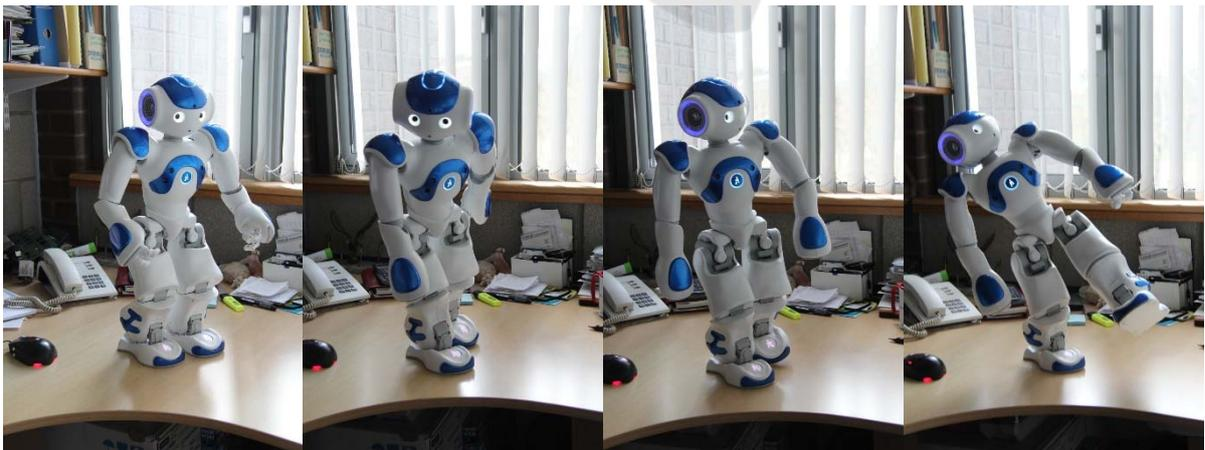
Figure 4: The evolved kick from Fig.3 as transferred to the real Nao robot. Compare these whole-body motions with the first four frames of Fig. 3.
