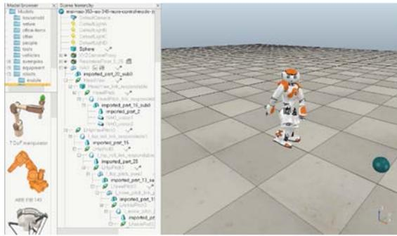
Figure 1: An example scene from the V-REP simulator. On the far left are examples of some of the robots that can be simulated, next to this is the scene hierarchy for the current scene, on the right is an example of an evolved kick.
