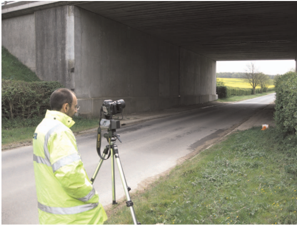
Figure 2. Prototype image collection system showing camera mounted on GigaPan unit
