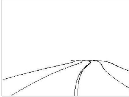
Fig. 4. Perspective projection of multi-lane road model.
