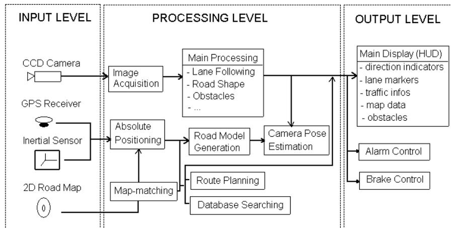
Fig. 1. System architecture of VICNAS.
