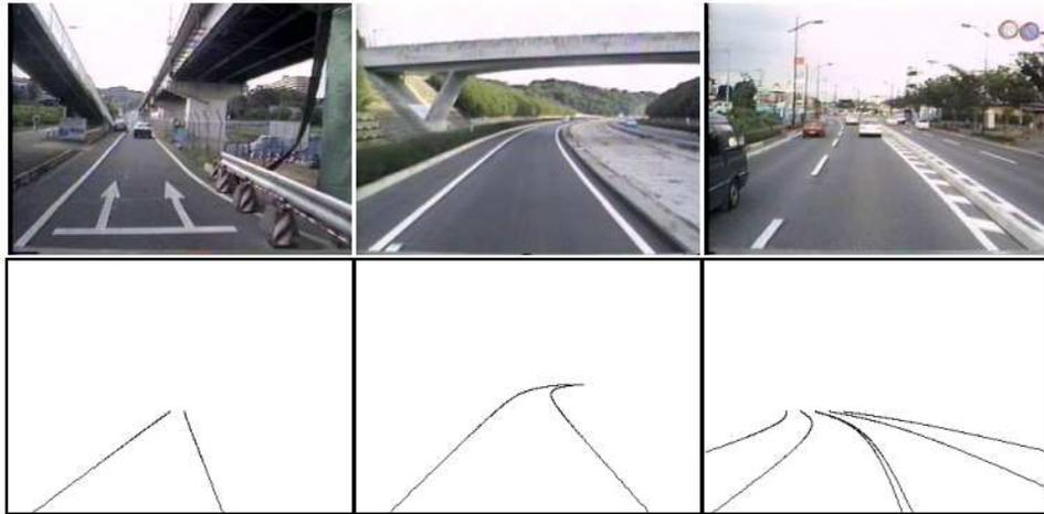
Fig. 7. Tested roads and road shape models.
