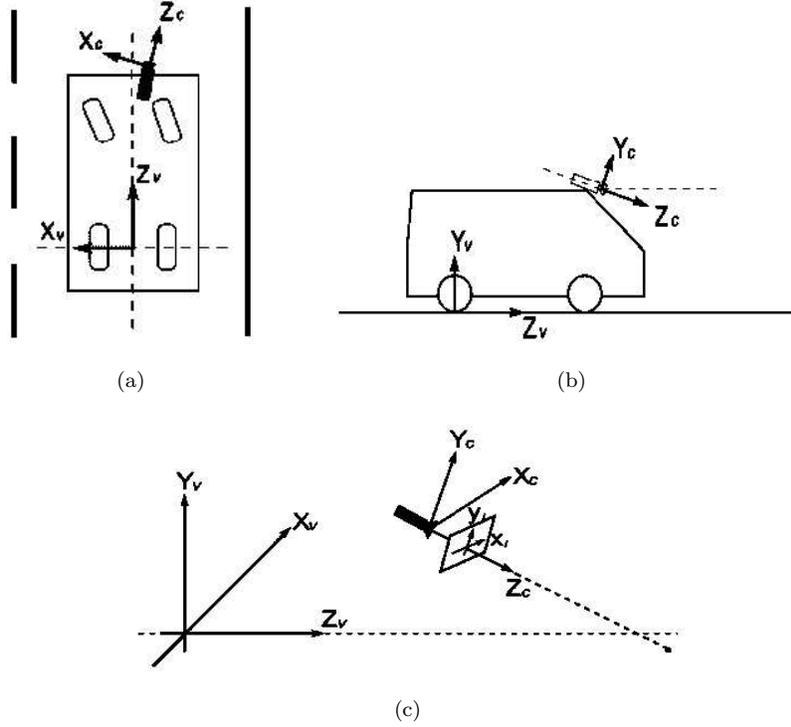
Fig. 2. The three reference frames of on-road navigation.
