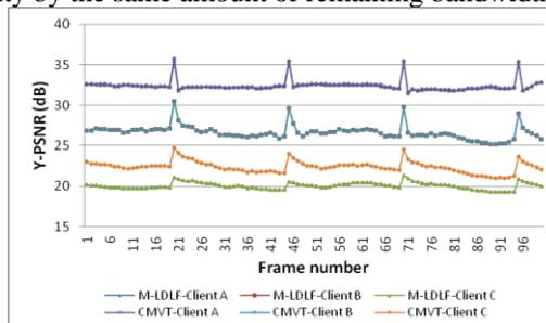
Figure 5. The Y-PSNR results of reconstructed video when using CMVT and M-LDLF.
