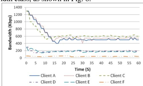
(a) Bandwidth adjustment using M-LDLF.
