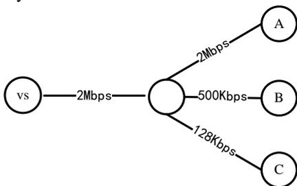
Figure 3. Clients A, B and C connect to the video server with different available bandwidth.
