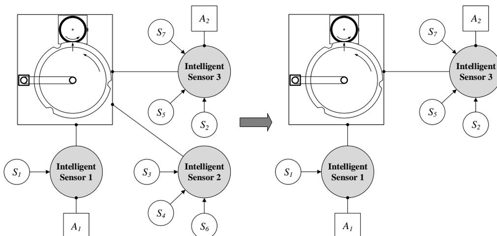
Figure 7. Rejection of one intelligent sensor from the fusion system architecture.
