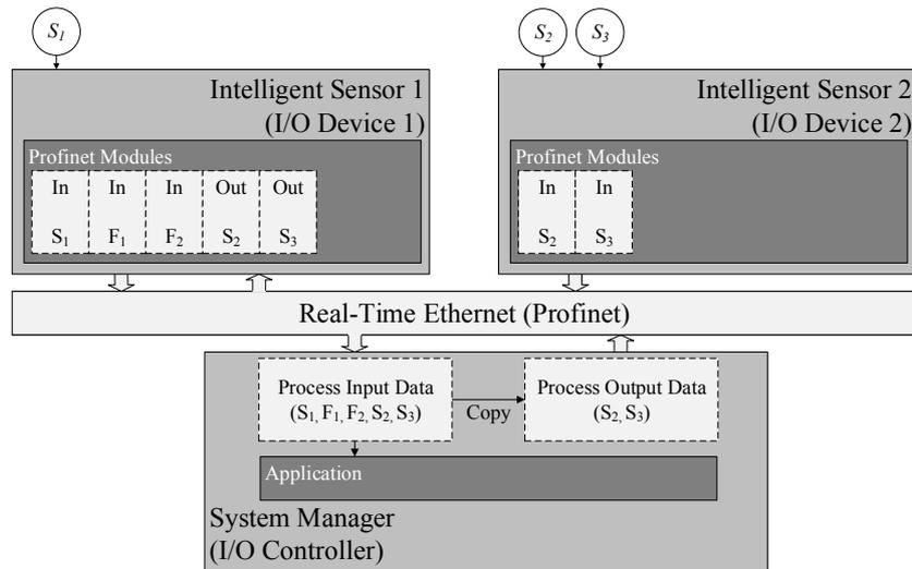
Figure 5. Profinet configuration of intelligent sensors in the fusion system network.
