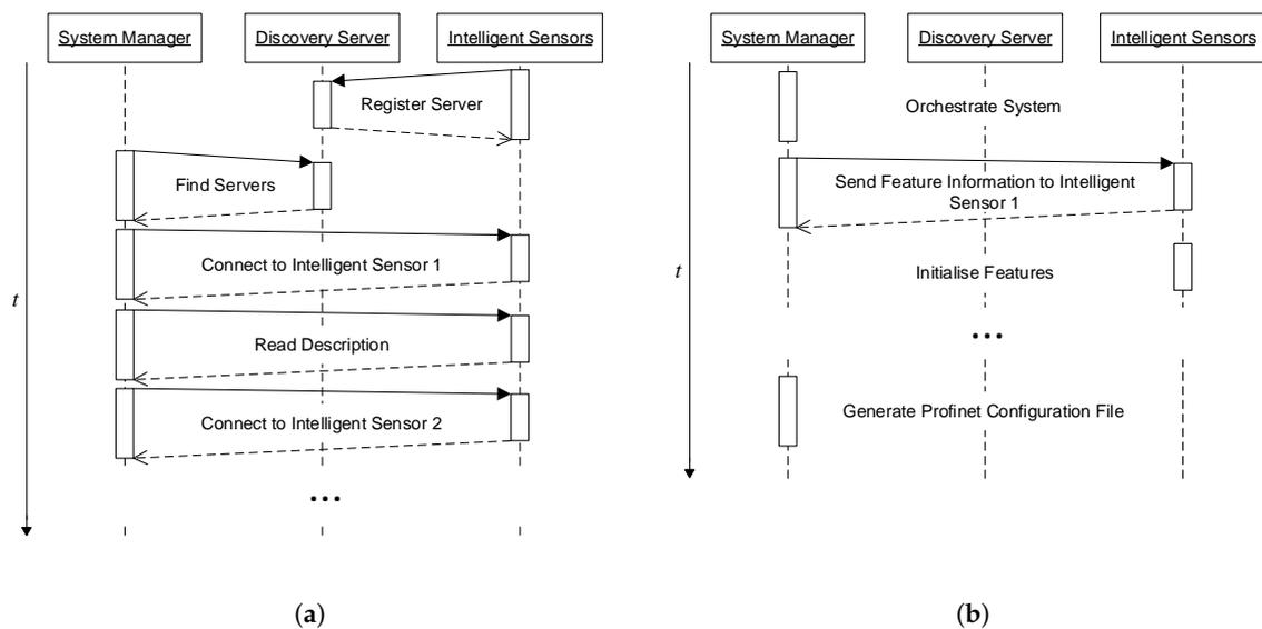
**Figure 4.** Communication sequences between system manager, discovery server, and intelligent sensors for SEFU/IFU system configuration. (a) Sequence describing the detection of intelligent sensors [52]; (b) Communication of feature information for assigning feature computation tasks to intelligent sensors.
