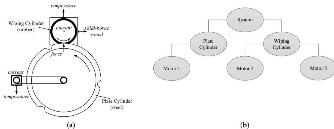
**Figure 6.** Set-up of the printing unit demonstrator. (a) Structural design of the printing unit demonstrator [6]; (b) Hierarchy of the demonstrator [7].
