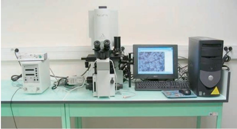
Figure 7.1 Laser capture microdissection (LCM) apparatus (Pixcell II from Arcturus).
