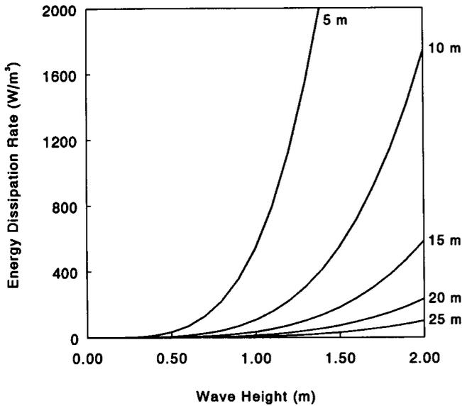
Figure 2. Energy dissipation rates in the benthic boundary layer. Predicted values given typical wave heights and water depths of habitats favored by *Strongylocentrotus purpuratus*. The wave period is assumed to be 10 s.
