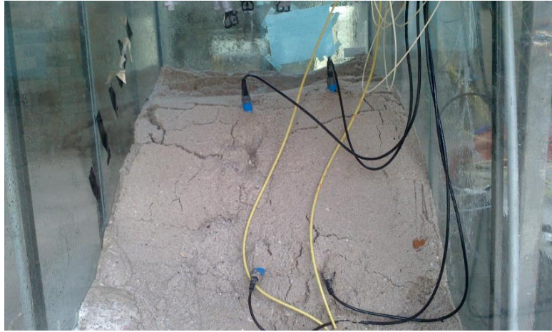
Figure 17. Slope failure (flowslide).
