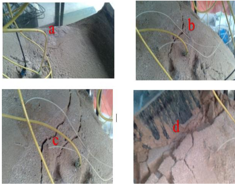
Figure 9. Failure events before the flowslide.
