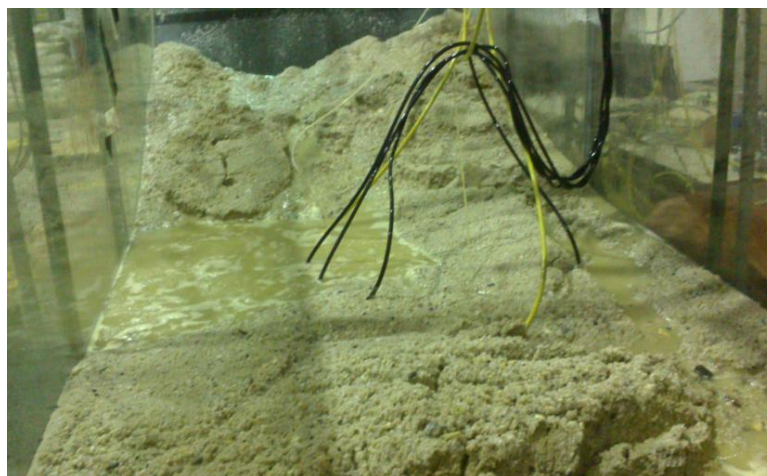
Figure 14. Slope failure (flowslide).
