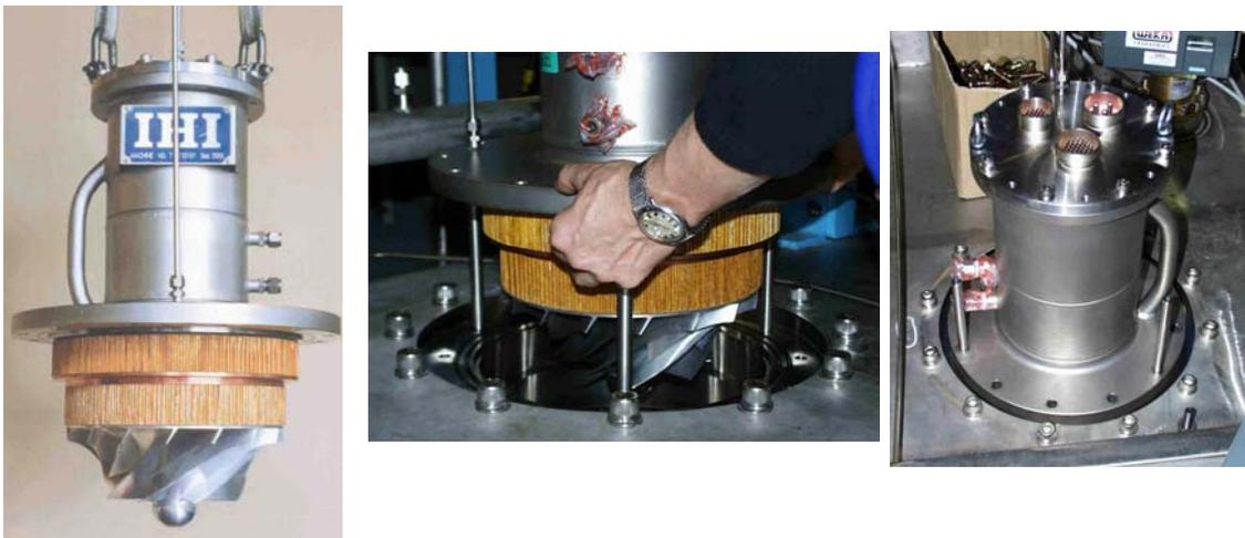
**FIGURE 8.** Cartridge handling (left), mechanical installation (middle) and utility plugging (right)
