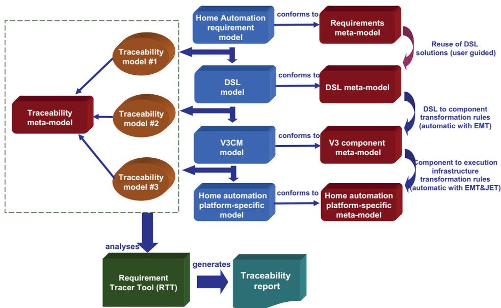
Figure 1: Framework for home automation model driven development.
