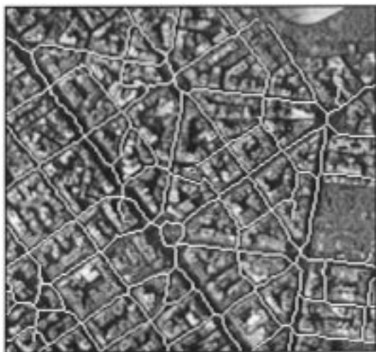
Fig. 6. Extracted road network overlapped with the original image of Athens.
