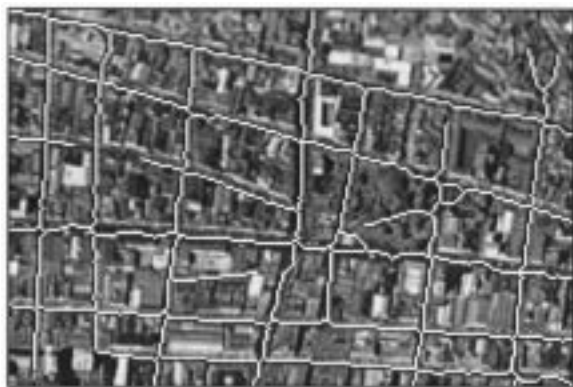
Fig. 5. Overlay of the extracted road network on the top of the original image of Valparaiso shown in Fig. 1.
