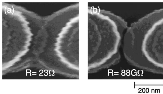
FIG. 1. Field-emission scanning electron micrographs of a representative gold nanowire (a) before and (b) after the breaking procedure. The nanowire consists of thin ( $\sim 10$  nm) and thick ( $\sim 90$  nm) gold regions. In the images, diffuse white lines separate these two regions.
