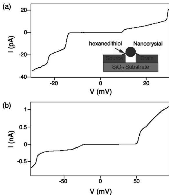
FIG. 3. Current vs voltage curves at  $T=1.5$  K obtained from single-electron transistors based on (a) 5 nm CdSe nanocrystals and (b) 7 nm CdSe nanocrystals. The inset in (a) shows the schematic diagram of an idealized device.
